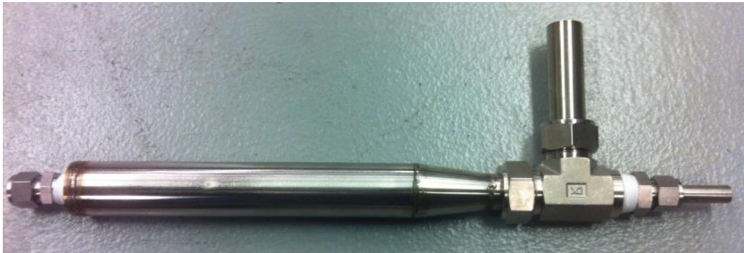
Figure 40 Pressure reducer fabricated for use on FI test stand
