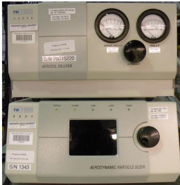
Figure 39 TSI Model 3321 APS with diluter used with FI test stand
