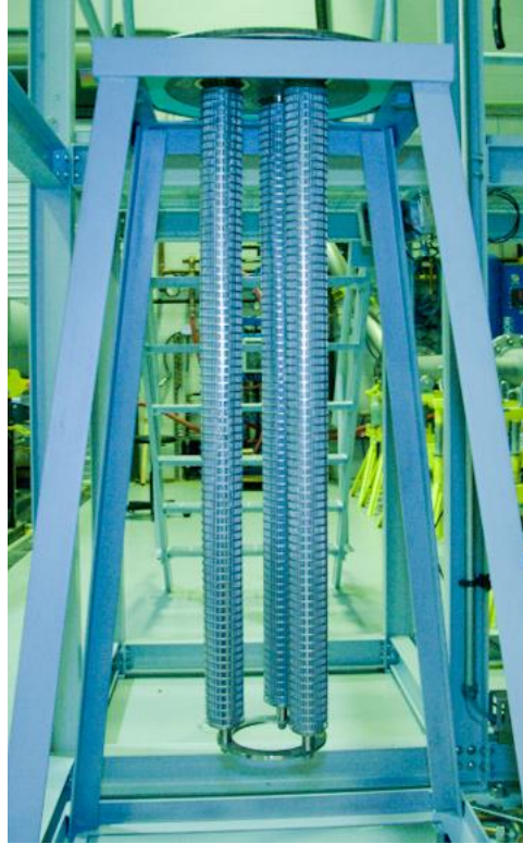
Figure 11 Porvair sintered metal media Section FI HEPA filter elements attached to the tubesheet
