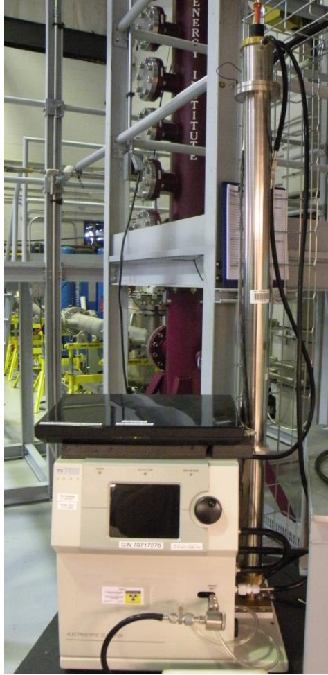
Figure 38 TSI Model 3080 Electro Static Classifier with Custom 37.4inch (95 cm) DMA used on FI test stand
