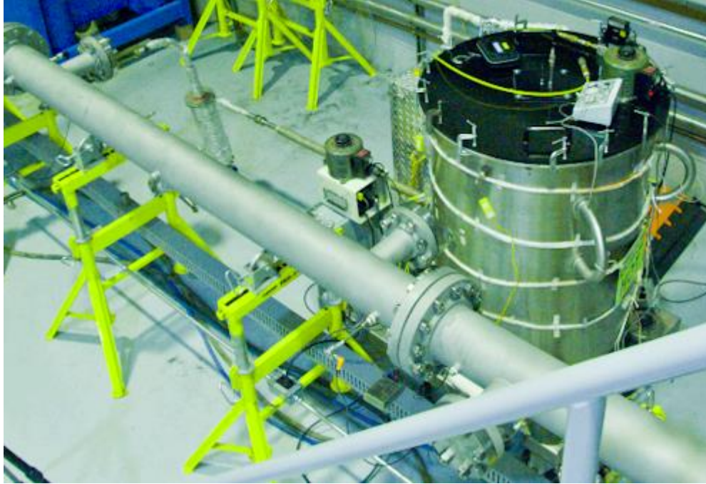
Figure 35 Stainless steel spray vessel and heater system for generating spray dried aerosols used in characterization testing
